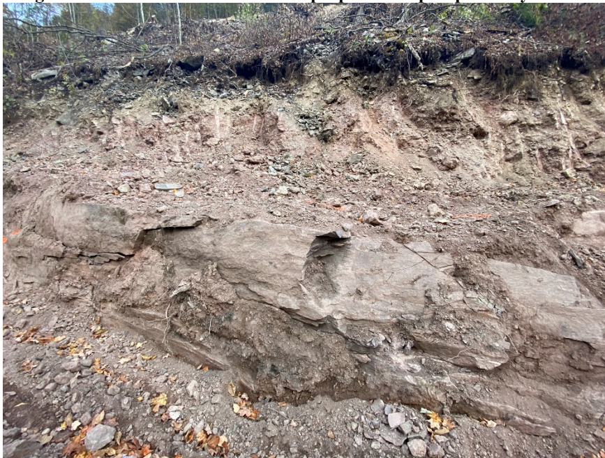
Image 9: View of sandstone at base of proposed steep slope at Loyalsock State Forest
