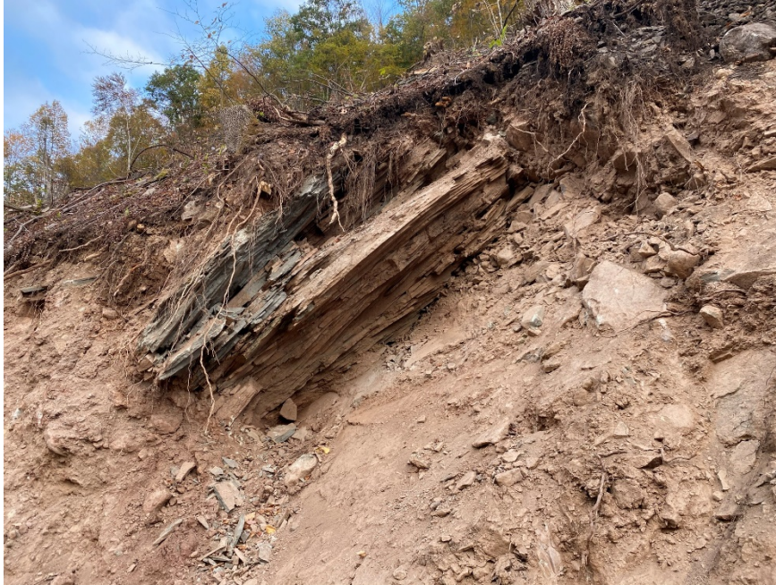
Image 8: View of steeply dipping interbedded sandstone and siltstone at the base of a proposed steep slope at Loyalsock State Forest
